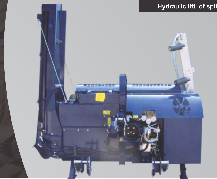
Hydraulic lift of splitting wedges made of Hardox 450
